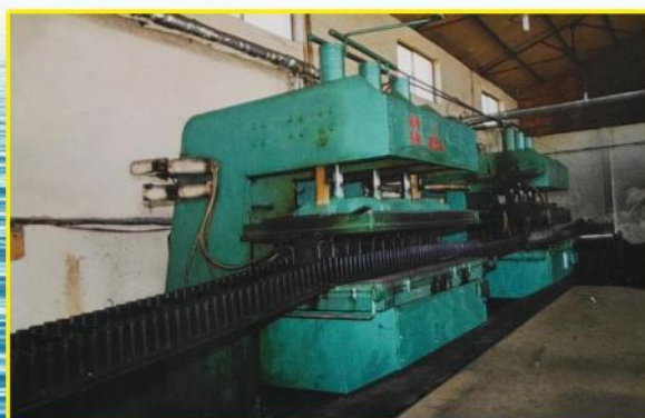
具有国内先进水平、生产宽2000mm挡边高500mm波状挡边带生产线 With the domestic advanced level, the production of wide ribs 2000mm high 500mm corrugated sidewall belt production line
